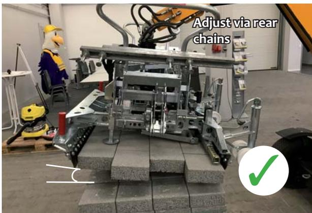
1. The stone formations 1 – 20 shown below are suitable among others for mechanical installation. Other stone formations can also be laid by machines as long as the stones are packed in the correct formation ready for the machine to lay them.
