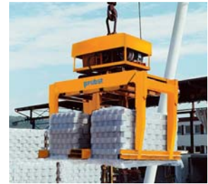
Double Grab STAZ-DZ-I, fixed to Overhead Crane
