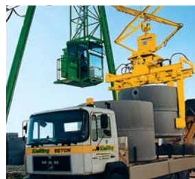
Manhole Ring Handling Systems RKUS
