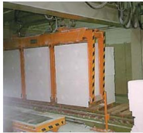
Cube Clamp STAZ with Hydraulic Divider
