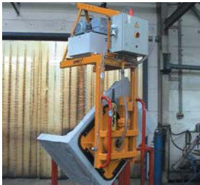
Vacuum Lifting Device with 180° Turning Unit
