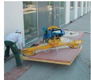
SH-2500-UNI with Spreader Bar
