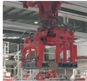
Hydraulic Cubing Clamp with Rotating Grippers – Rotating Range 180°
