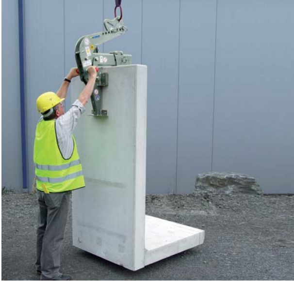
Grab for Angular Concrete Products WEZ-2
