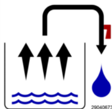
Drain condensed water daily 2904.0673
