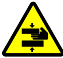
Warning Crushing hazard to hands 2904.0396
