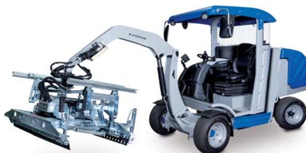
Entry-level model with partially enclosed operator's cabin, adjustable standard seat with mechanical suspension, 2.4" screen and standard boom.
