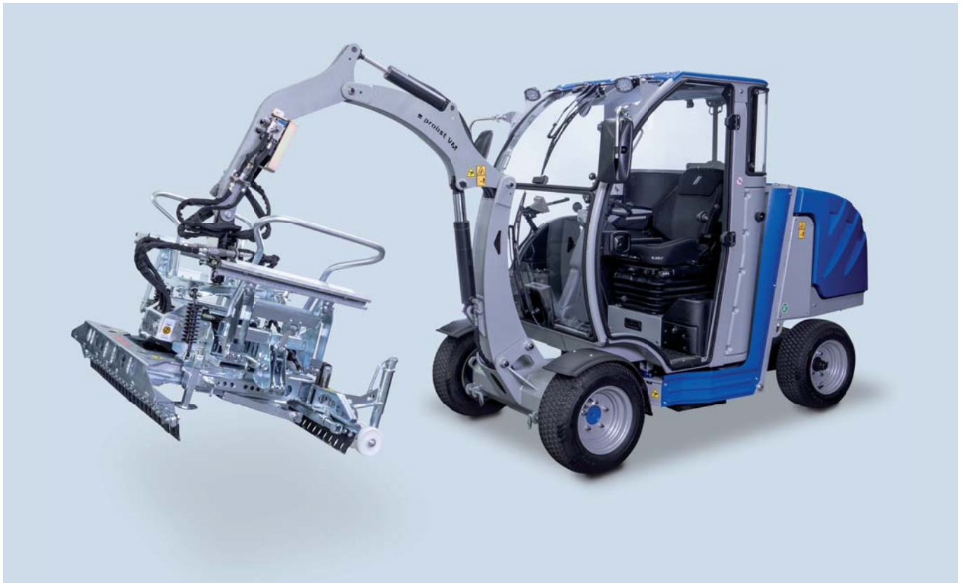
VM-X-PAVERMAX premium with HVZ-UNI-II (picture with accessories LED light package and exterior mirrors)
