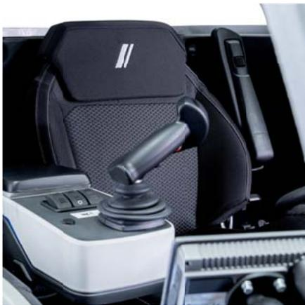
Joystick with ergonomically arranged controls
