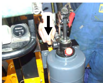
Stellhebel an Handpumpe in Position I bringen
