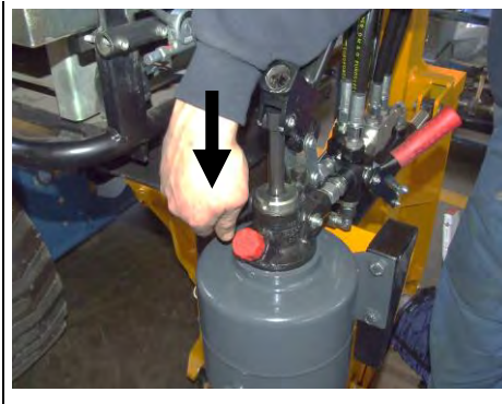
Stellhebel an Handpumpe in Position II bringen
