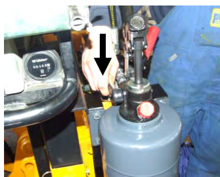
Stellhebel an Handpumpe in Position I bringen
