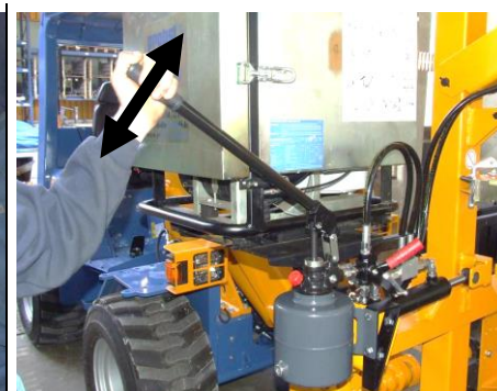
Actuating the hand pump moves the mast to the left.
