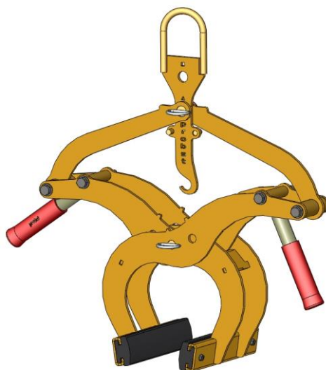
Gripping position of the device (with load)
